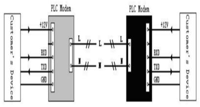
Figure 2: Application Diagram of PLC modem
